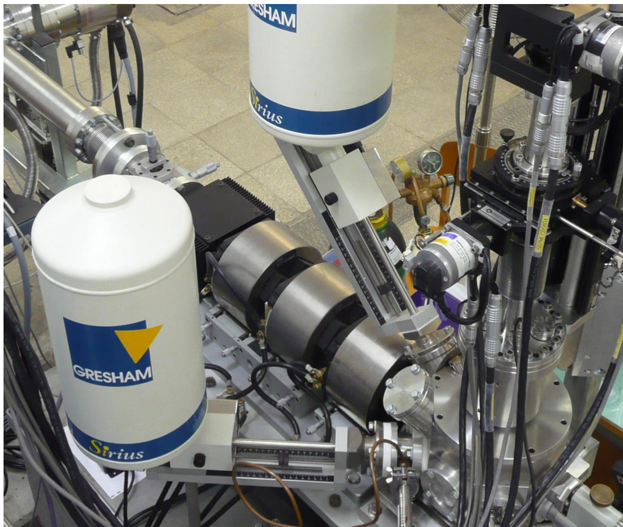
Figure 1: The ATOMKI-HAS Oxford-type nuclear microprobe. The sample chamber is equipped with a 5-axis goniometer, 2 X-ray detectors and particle detectors making available high lateral resolution elemental analysis simultaneously.
